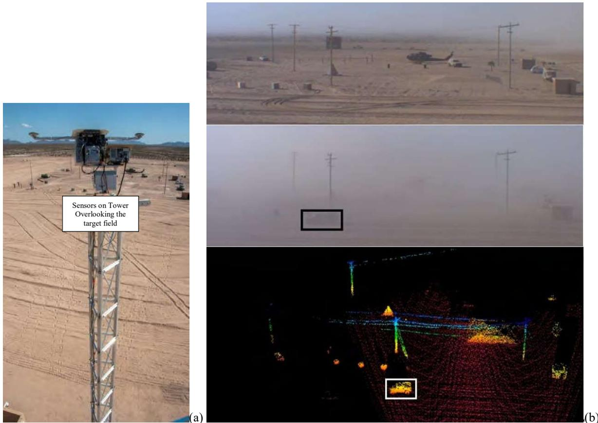
Figure 9. (a) Picture of the OPAL-DRP installed on a tower. (b) The two video images at the top compare the scene in absence and in presence of dust. The OPAL-DRP LiDAR image at the bottom has been obtained at the same time as the image obscured by the presence of dust. The OPAL-DRP was set at a fix position while performing a horizontal scan operating at 25 kHz. The vehicle shown into the rectangle was absent from the clear scene.
