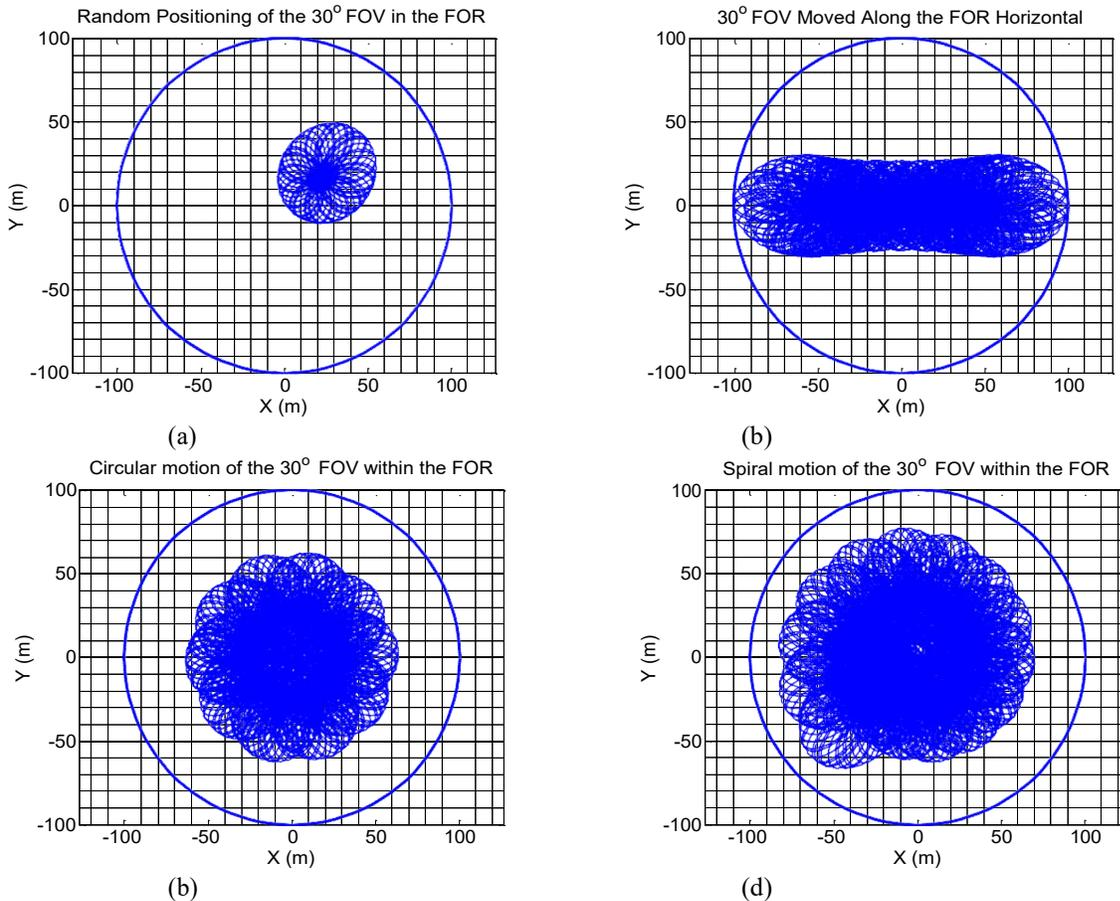
Figure 4. Examples of simple scan scenarios where a  $30^\circ$  FOV is moved within a  $90^\circ$  FOR.
