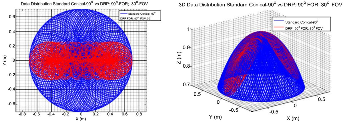
Figure 5. Comparative data density distribution between a standard conical Risley prism scanner and the DRP using the small FOV along the horizontal.
