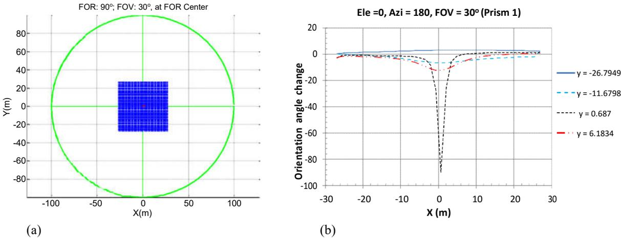
Figure 1. (a) Small focused raster scan FOV area generated by a single prism pair. (b) Corresponding change in angular position for prism #1 as a function of the data points coordinates.
