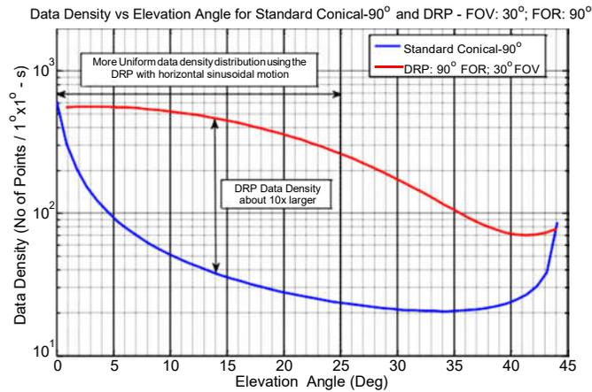
Figure 6. Comparative data density (No. of data points / 1°x1°-s) versus elevation angle for a standard conical Risley prism scanner and the DRP moving a 30° FOV along the horizontal of a 90°FOR.
