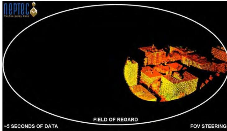
Figure 8. Data acquired with the DRP while the FOV is moved along the horizontal of the FOR.
