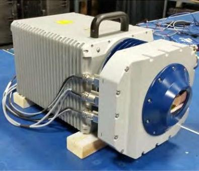
Figure 3. Picture of the Double Risley Prisms Pair implementation based on the Neptec's OPAL-ECR LiDAR.
