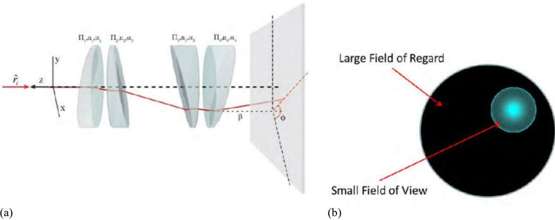
Figure 2 (a) Optical arrangement for the DRP system. (b) Illustration of a small FOV being moved into a larger FOR.
