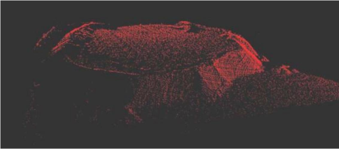
Fig. 7: Data combined from two scanners showing a shadow area that was not covered by either scanner.
