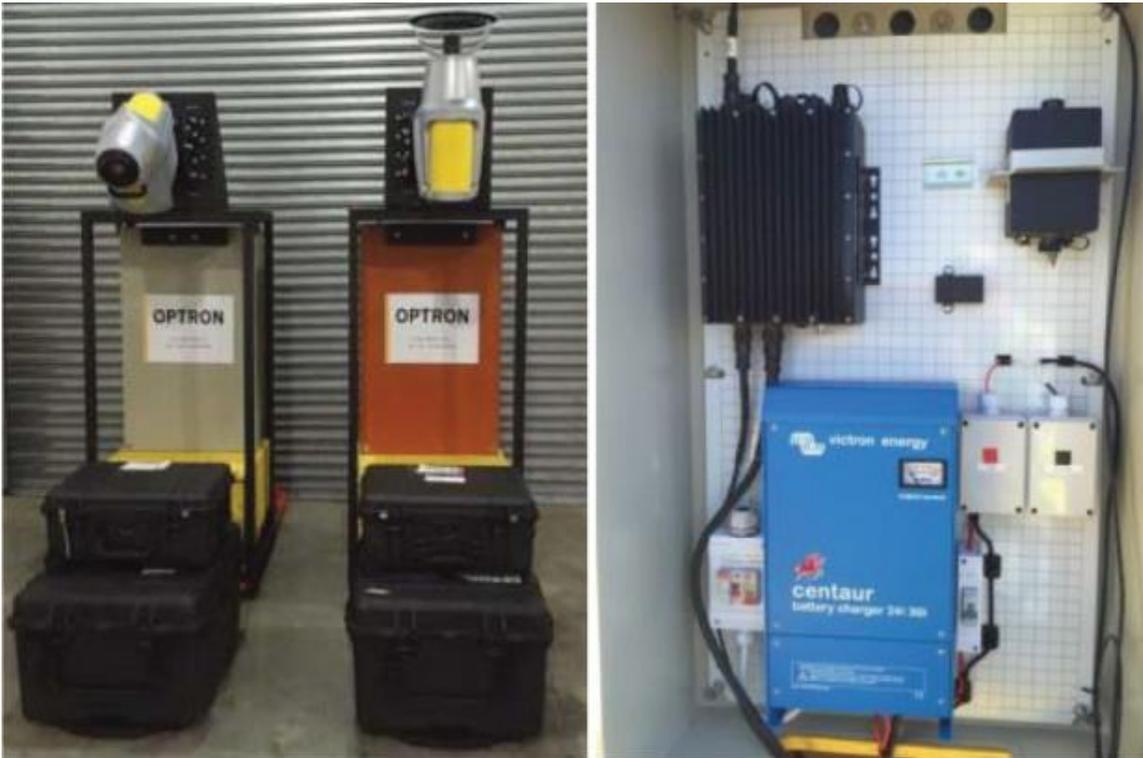
Fig. 4: Frame holding the scanners in position and a housing for batteries, battery charger and rugged computer running 3DRi software.
