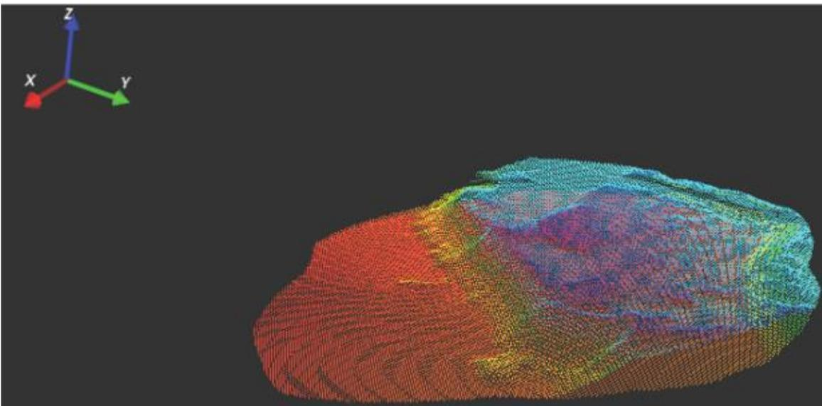
Fig. 9: The stockpile shown above the base or floor level, colour-coded according to elevation.
