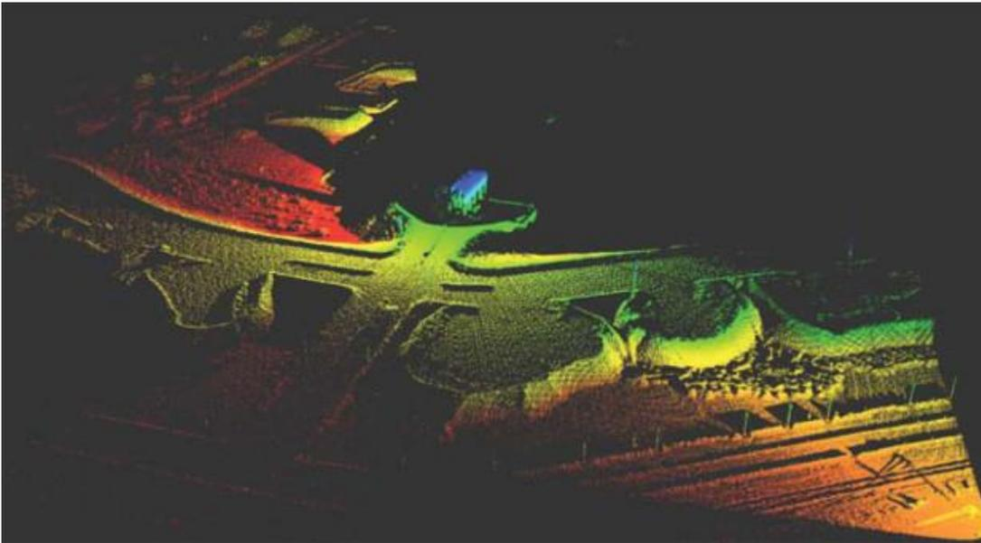
Fig. 6: Data combined from two scanners with five seconds of lidar data.
