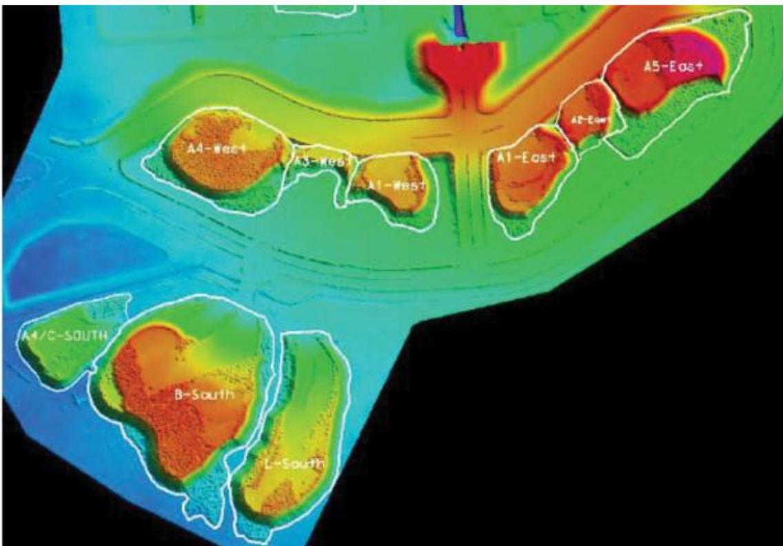
Fig. 10: Aerial lidar relief map from April 2015, note the boundary between A2-east and A5-east and how it differs in Fig. 11, as well as the many small piles.
